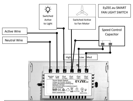
Some common capacitor wiring colour schemes used in AU/NZ (Electrician guide only) **BRAND** (1)HIGH (2)MED (3)LOW SPEED>> **HPM Vivo** Blue Grey Orange DETA/Clipsal/Schneider Red **Purple** Orange Supplied with switch Red Blue **Black** NOTE: All electrical installation must be completed by registered electrician NOTE: Faceplate is reversable so Light/High/Med/Low order may be reversed
